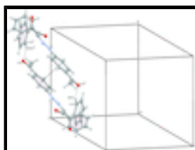
Fig. 2. Part of the crystal packing showing the formation of an inversion-related dimer via C15—H15 \cdots O3 i weak contacts (dashed lines) and a \pi - \pi stacking interaction (solid line) [symmetry code: (i) -x + 2, -y + 1, -z ].
